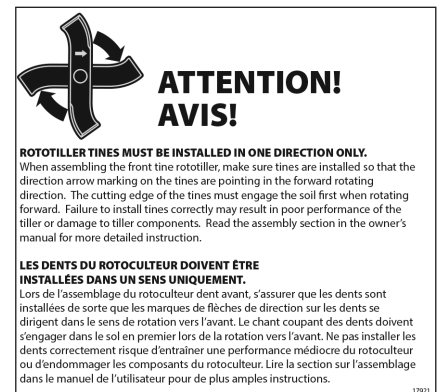
Part No. 17920 CORRECT TINE INSTALLATION
